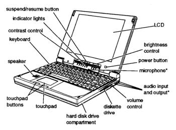
These parts function only with the optional audio card installed.
